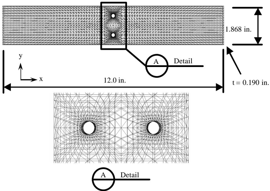
Figure 2: Finite element mesh for case study
