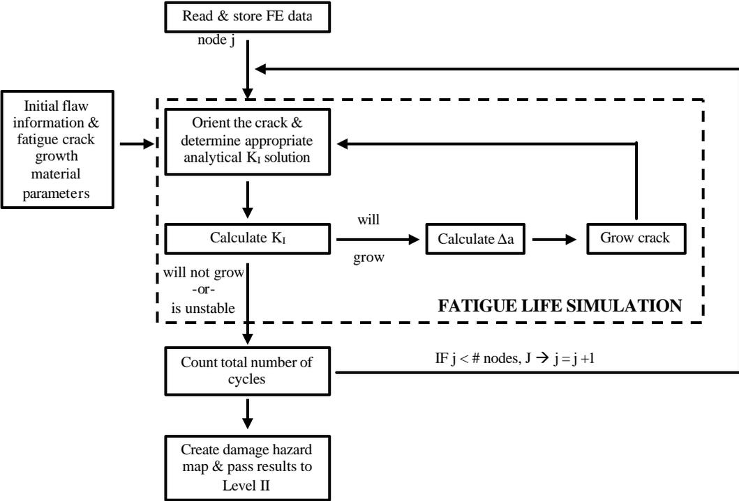
Figure 1: Flowchart for DDSim Level I
