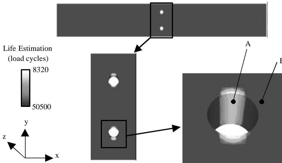
Figure 3: Damage hazard map for case study
