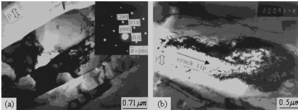
Figure 5: (a) Layered microstructure in Al interlayer and TEM diffraction patterns
