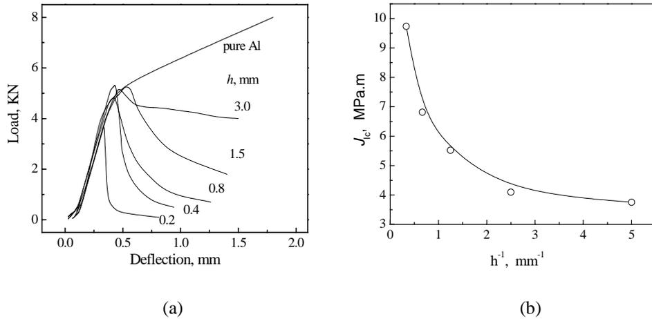
Figure1: Load-deflection curves (a) and critical integral (b) with interlayer thickness,  $h$
