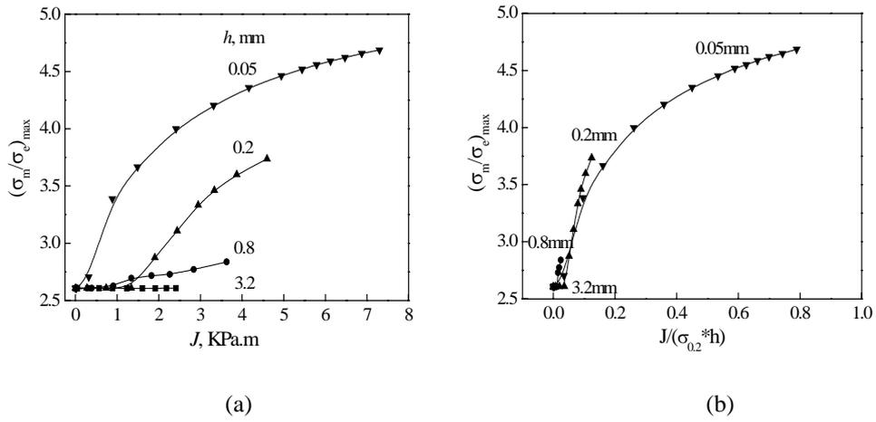
Figure 4: Peak stress triaxiality versus load characterized by  $J$  integral (a) and normalized  $J$  integral (b) respectively
