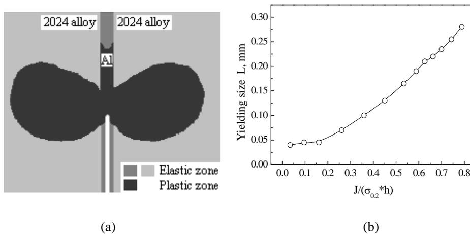
Figure 3: Plastic zone in Al interlayer,  $h = 50 \mu m$ , constrained by neighboring elastic substrates (a) and its size growing in the direction of interfaces (b)
