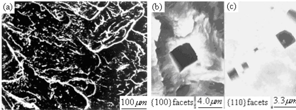
Figure 2: Typical river patterns (a), {100} cube-shaped etch pits (b) and {110} symmetrical V-notch shaped etch pits (c)
