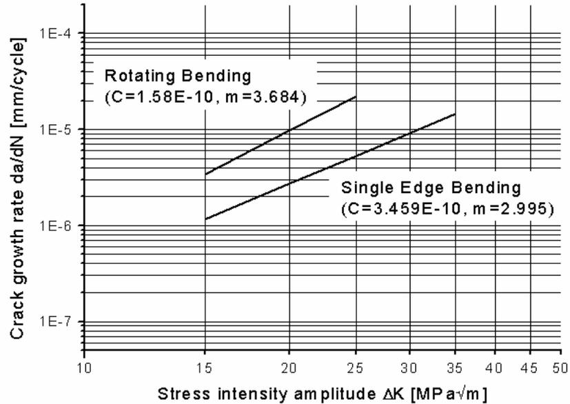
Figure 5: Comparison of the crack growth behavior in rotating bending tests and single edge notch beam bending tests
