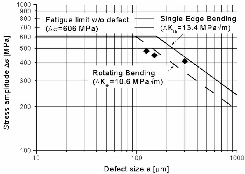
Figure 4: Fatigue limit diagram: comparison of rotating bending tests (data points and dashed mean curve) and single edge notch beam bending tests (full line)
