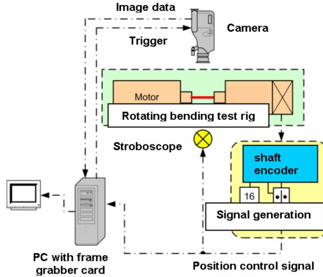
Figure 3: Experimental setup
