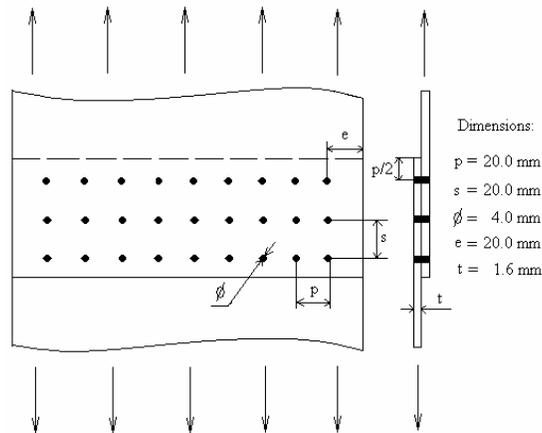
Figure 1: Lap joint configuration.
