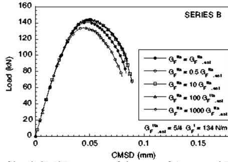
Figure 3: Numerical predictions of load-CMSD curves of the test of Arrea and Ingraffea [2], with  $G_F^{IIa} = 0.5, 1, 10, 100$  and  $1000 G_F^I$ .
