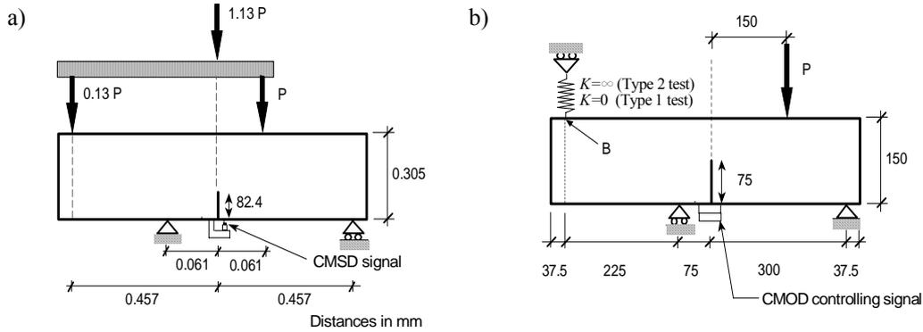
Figure 2: Geometry, forces and boundary conditions of the tests of: a) Arrea and Ingraffea [2], and b) Gálvez *et al.* [13].
