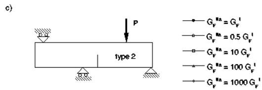
Figure 4: Numerical predictions of the *type 1* tests of Gálvez et al. [13], with  $G_F^{IIa} = 0.5, 1, 10, 100$  and  $1000 G_F^I$ : a) load-CMOD, b) load-displacement, c) legend and scheme.
