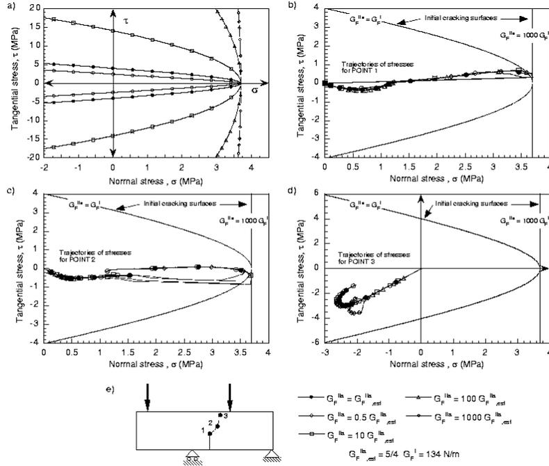
Figure 6: Initial cracking surfaces and numerical trajectories of the stresses in the crack with  $G_F^{IIa} = 0.5, 1, 10, 100$  and  $1000 G_F^I$  during the tests of Arrea and Ingraffea [2]: a) initial cracking surfaces. Trajectories of the stresses in the crack for: b) start of the crack (point 1), c) middle of the crack path (point 2) and d) near the end of the crack path on the uncracked ligament (point 3). e) scheme of the specimen and legend.
