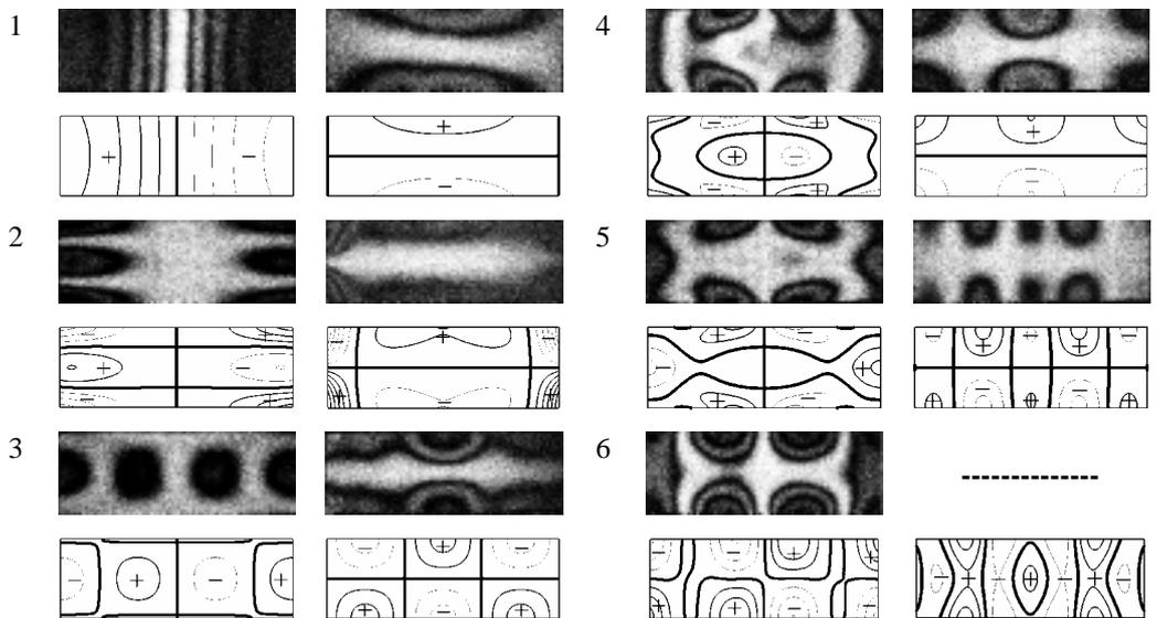
Figure 3: The in-plane mode shapes of the GFRP piezolaminated composite plate obtained by AF-ESPI and FEM.
