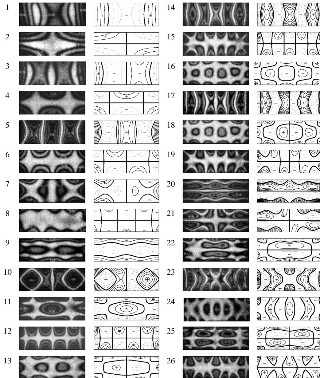
Figure 1 :The out-of-plane mode shapes of the thin piezoceramic plate obtained by AF-ESPI and FEM
