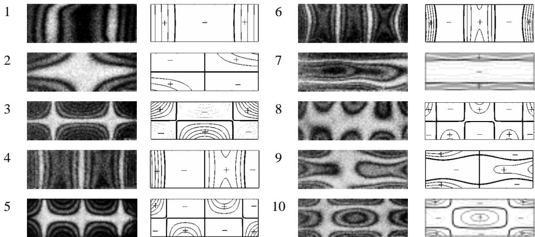
Figure 2: The out-of-plane mode shapes of the GFRP piezolaminated composite plate obtained by AF-ESPI and FEM.
