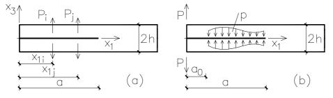
Figure 1: Schematic of the DCB specimen under different loading conditions.
