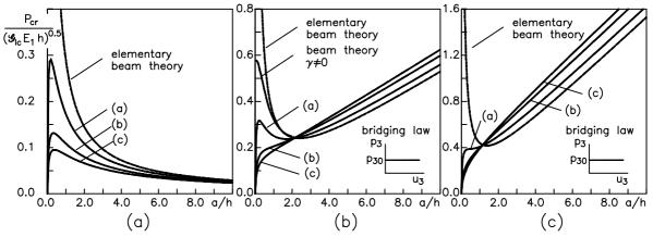
Figure 2: Dimensionless critical load versus normalized crack length in orthotropic DCB specimens. (a) No bridging. (b) Bridging tractions  $p_3 = 0.1 \sqrt{G_{Ic}E_1/h}$ . (c) Bridging tractions  $p_3 = 0.3 \sqrt{G_{Ic}E_1/h}$ .
