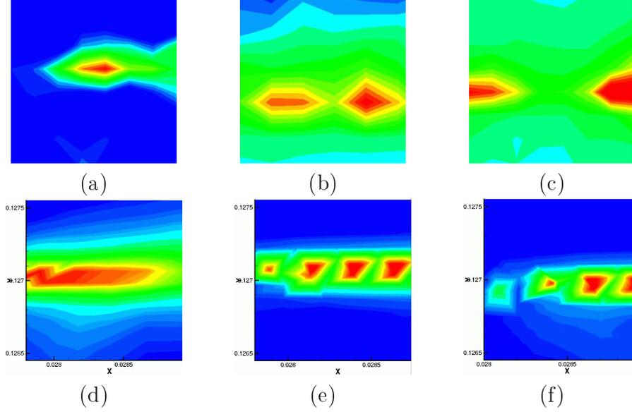
Fig. 2. Qualitative comparisons between experimental data and numerical computation on temperature distribution within the shear band ( $V = 37m/s$ ): (a),(d)  $t = 12\mu s$ ; (b),(e)  $t = 36\mu s$ ; (c), (f)  $t = 72\mu s$ ; (Experimental results : (a,b,c); Numerical results :(d,e,f) ).
