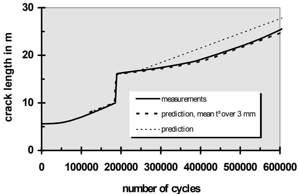
Figure 4. Measurements and prediction of the a-N curve in AA 2024 with 5000 underloads, underload sequence  $\Delta K=5-16-5$  (MPa $\sqrt{\text{cm}}$ ) at  $K_{\text{max}} = 29$  (MPa $\sqrt{\text{cm}}$ ) and 10 Hz.
