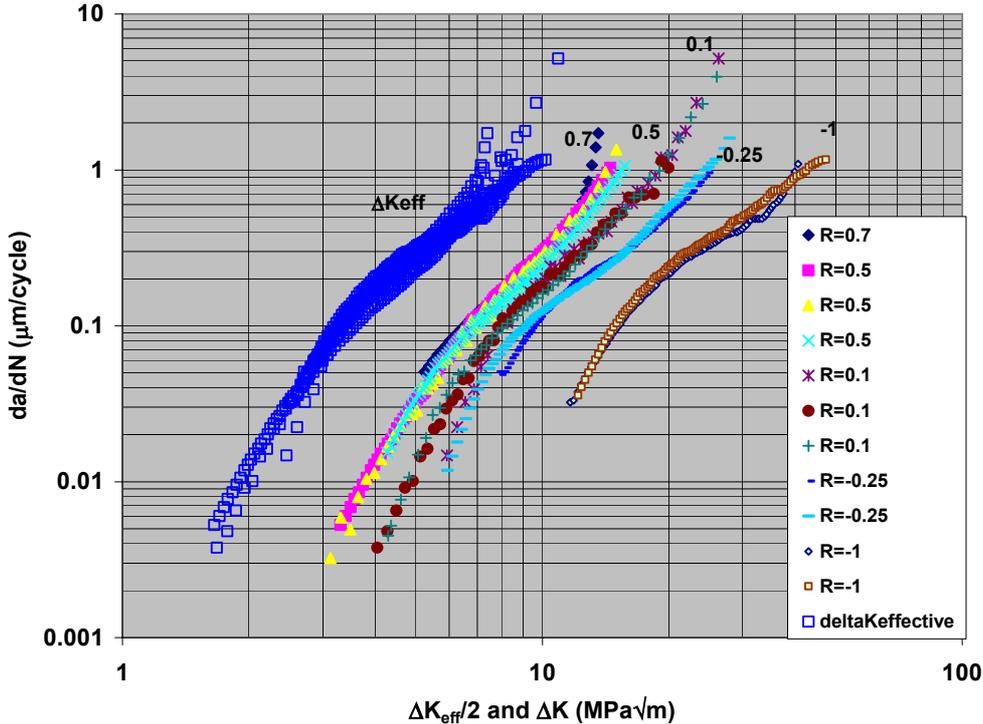
Figure 1. Results of 11 constant amplitude tests on AA 5083 at 5 different values of R and the corresponding  $da/dN$ - $\Delta K_{\text{eff}}$  (shifted a factor 2 to the left for clearness).
