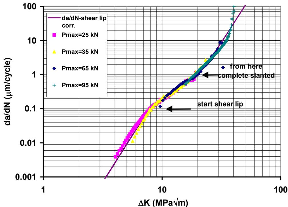
Figure 3 Experimental fatigue crack growth rate results and prediction for AA5083 at R=0.1
