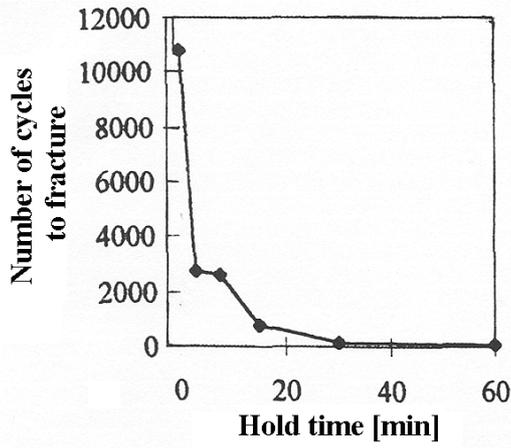
**Figure 3:** The dependence of hold time on the number of cycles to failure
